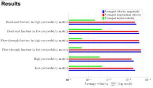
Average Velocity magnitude, average longitudinal velocities, and average lateral velocities of low- and high-permeability matrices as well as embedded dead-end and flow-through fractures.
