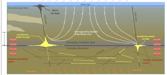
Figure 1 :Conceptual model showing at least two main available flow mixing paths created by invading evaporitic brines.
