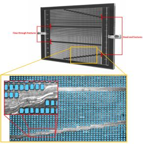
A time-lapse image of particle trajectories, captured during a time interval of 25 sec. The whiteness quantifies the particle density. Blue patches indicate the masks which are applied to exclude regions of impermeable pillars during the PIV calculations.
