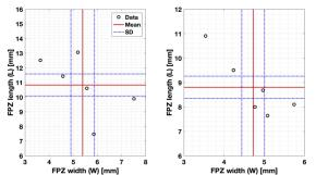
Figure 5: The measured values for the FPZ width (W) and length (L) for two cases of  $\phi = 0^{\circ}$  and  $\phi = 90^{\circ}$ . The mean values of the six tests are shown by red line, while the blue pointed line show the standard deviation. The results are taken from the fully formed FPZ, i.e. at 70% of pre-peak load for  $\phi = 0^{\circ}$  and 90% of pre-peak load for  $\phi = 0^{\circ}$  and 90% of pre-peak load for  $\phi = 0^{\circ}$  (Dutler et al., 2016).
