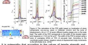
It is noteworthy that according to the values of tensile strength and Young's moduli, a critical tensile strain of about 270 and 350 micro strains are obtained for the principal directions normal and parallel to
