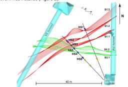
Figure 1: Experimental volume at GTS (top view): Injection boreholes (black lines), HF injection intervals (orange cylinders), HS injection intervals (blue cylinders), the shear zones along with the far field stress state ( $\alpha$ 1: ~ 13.8 MPa, plunging to the East with 30 – 40°,  $\alpha$ 3: ~ 8 MPa, subhorizontal North-South,  $\alpha_2 = \pi$  8.5 MPa, Krietsch et. al, 2018)
