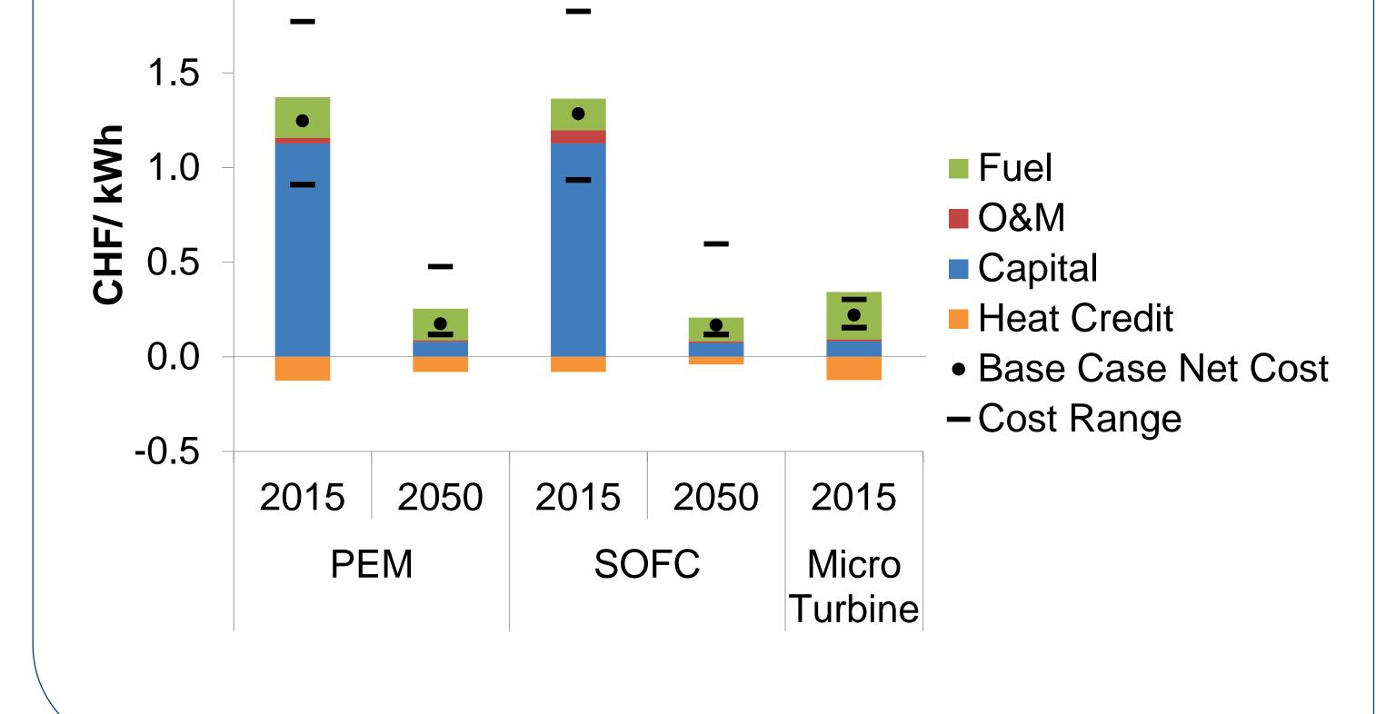
Particularly SOFCs are interesting due to their high efficiency, lack of platinum group metals and ability to easily reform lower purity fuels, such as biomethane.
