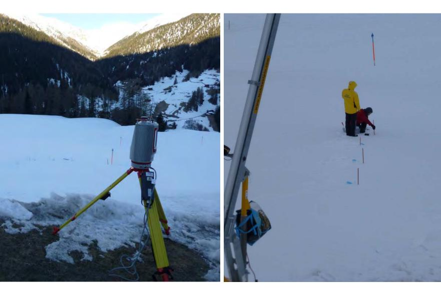
Figure 6: Terrestrial laser scanning (left) and manual snow observations (right) during snow making test
