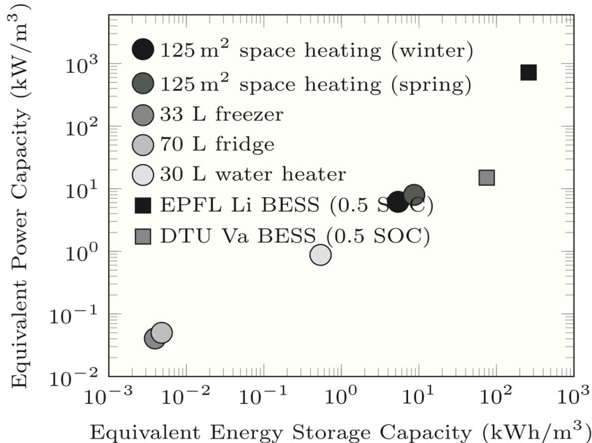
**Fig.: Storage capacity of reference TCLs vs reference battery systems.**
