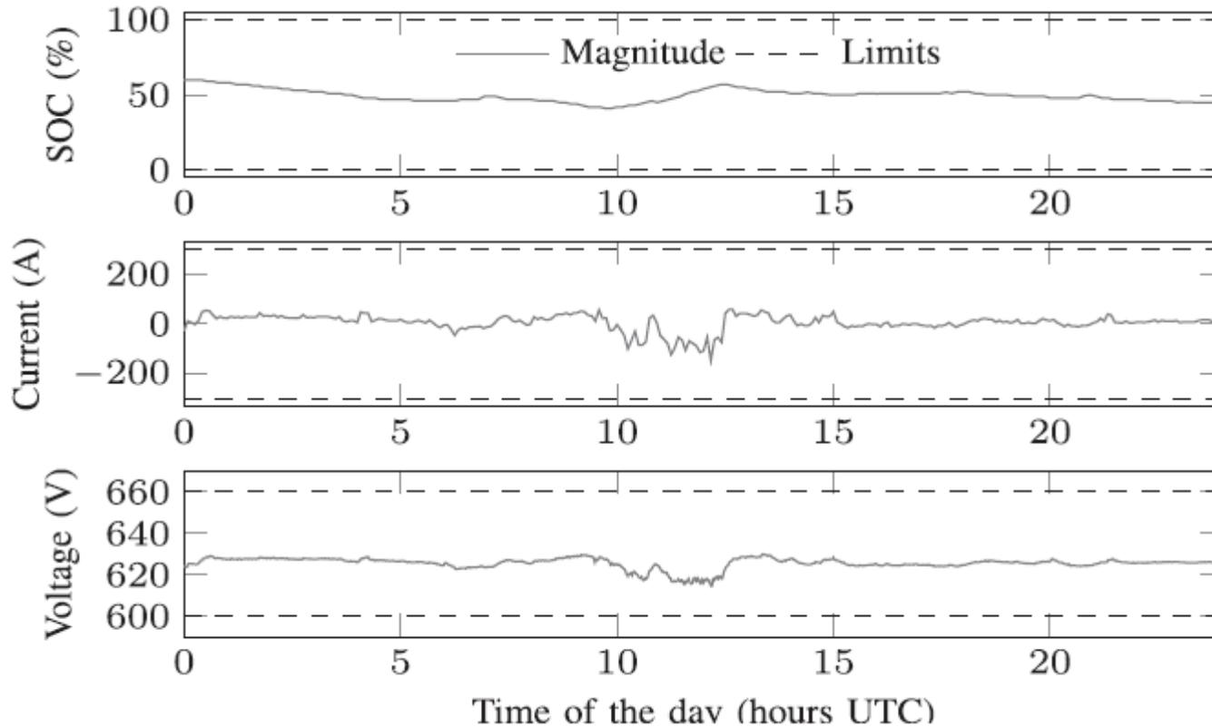
**BESS state-of-charge, DC Current and DC voltage with respective limits.**
