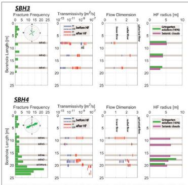
Figure 2. Profiles of fracture frequency, transmissivity, flow dimension, and the estimated radius of hydraulic fractures along the SBH3 (top) and SBH4 (bottom) boreholes. The location of each HF test is shown using the gray bands. Blue and red lines represent the value of hydraulic parameters before and after each HF test, respectively.
