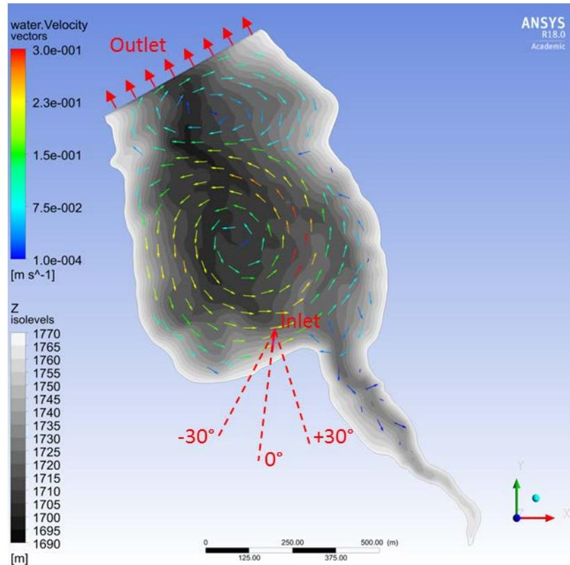
Flow velocity vectors at the water surface for  $Q = 90 \text{ m}^3/\text{s}$  and  $\alpha = 0^\circ$
