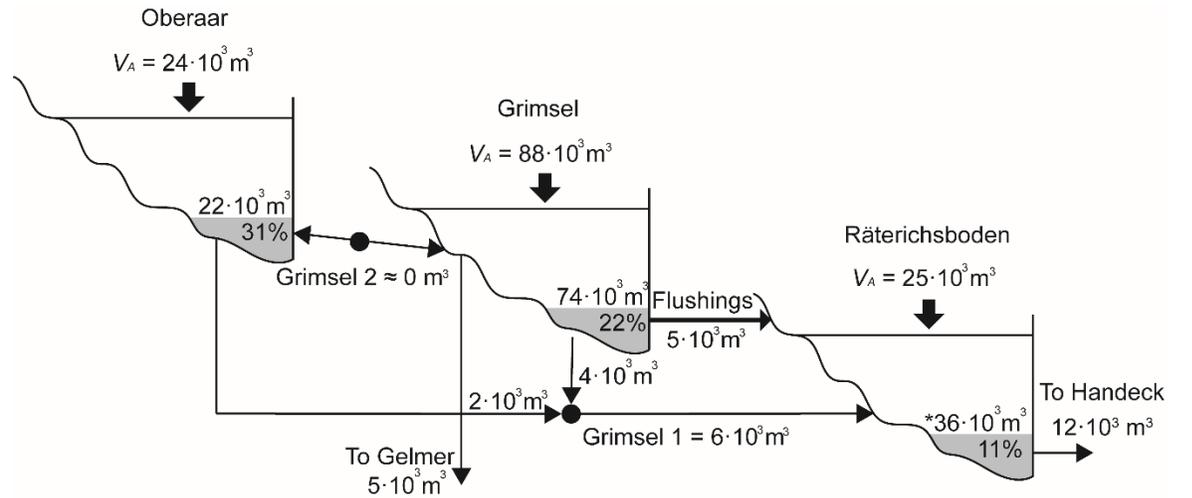
Sediment balance of the system of reservoirs in cascade
