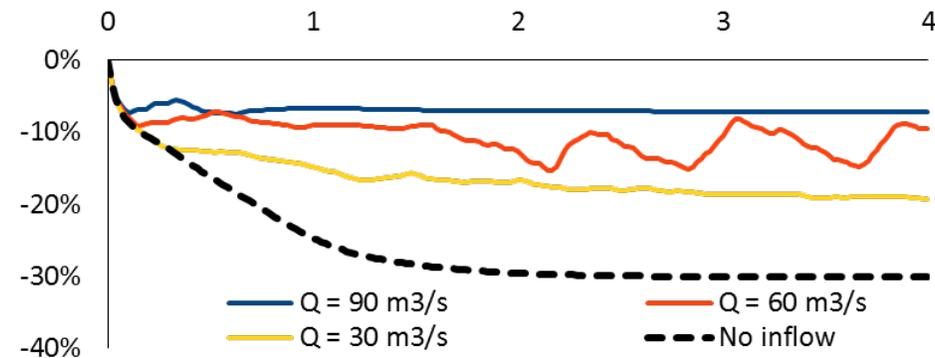
Deposition of fine sediments for different orientations and discharges of the jet-like inflow
