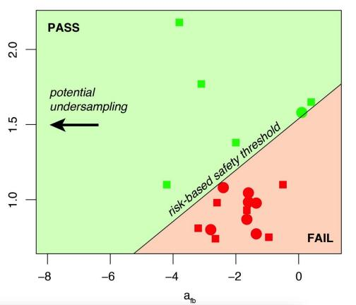
$\Pr(m \ge m_{saf}) = 1 - \exp\{-10^{a_{fb} - bm_{saf}} [V(t_{shut-in}) + \tau \dot{V}(t_{shut-in})]\} = Y$
